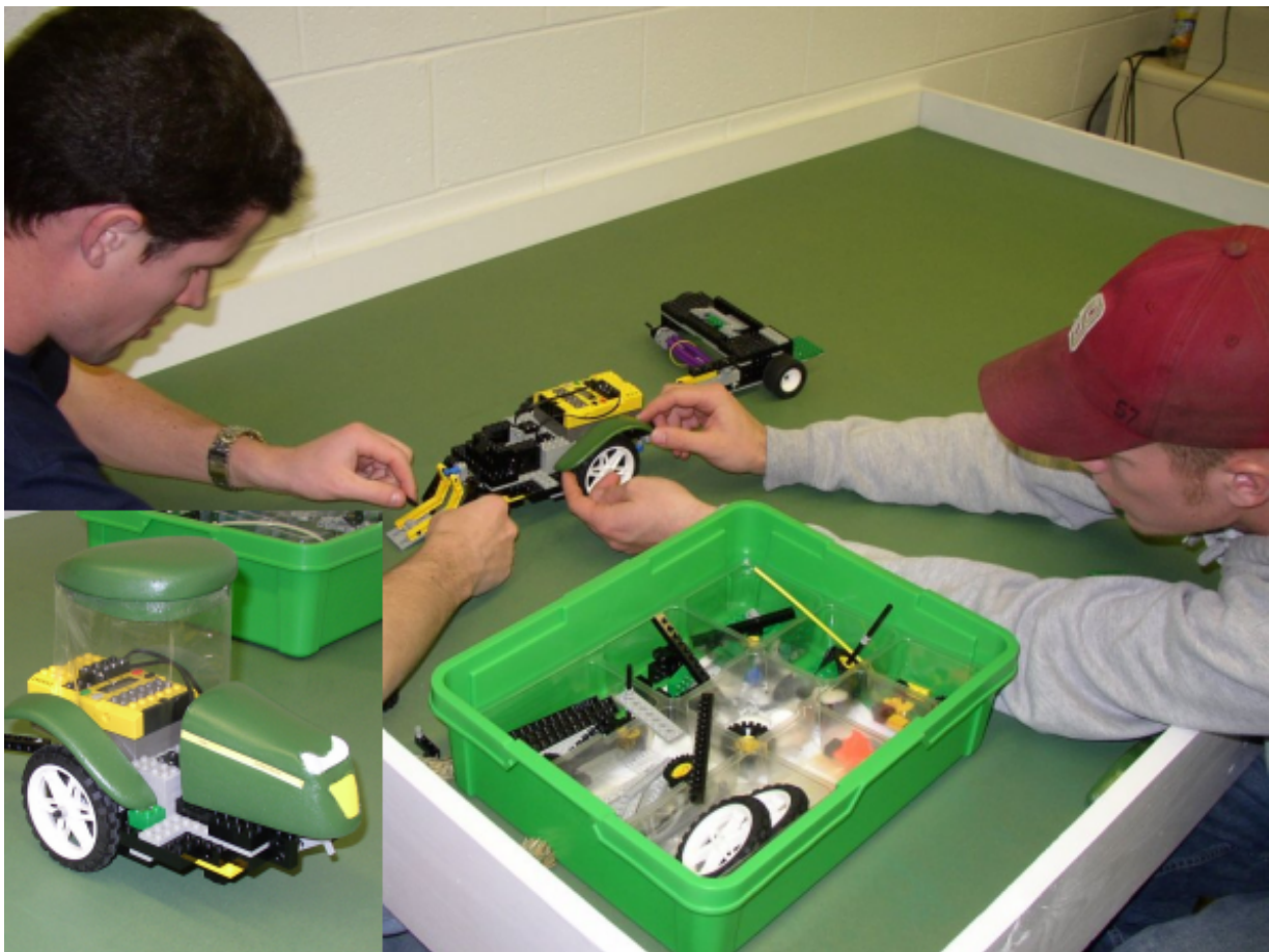
Figure 3 Group 3 developing an optimized system to steer an offset harvester through a 90 degree corner without leaving any crop standing
